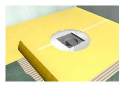
Step 1 The floor must be insulated with a suitable liquid waterproofing material.
